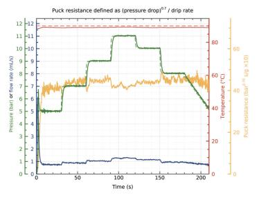
resistance of the gicleur with the resistance of the puck. Therefore, in a situation where the puck contributes little to the resistance, the system's resistance will tend toward that of the gicleur; in a situation where the puck contributes most, the system's resistance will tend toward that of the puck.
